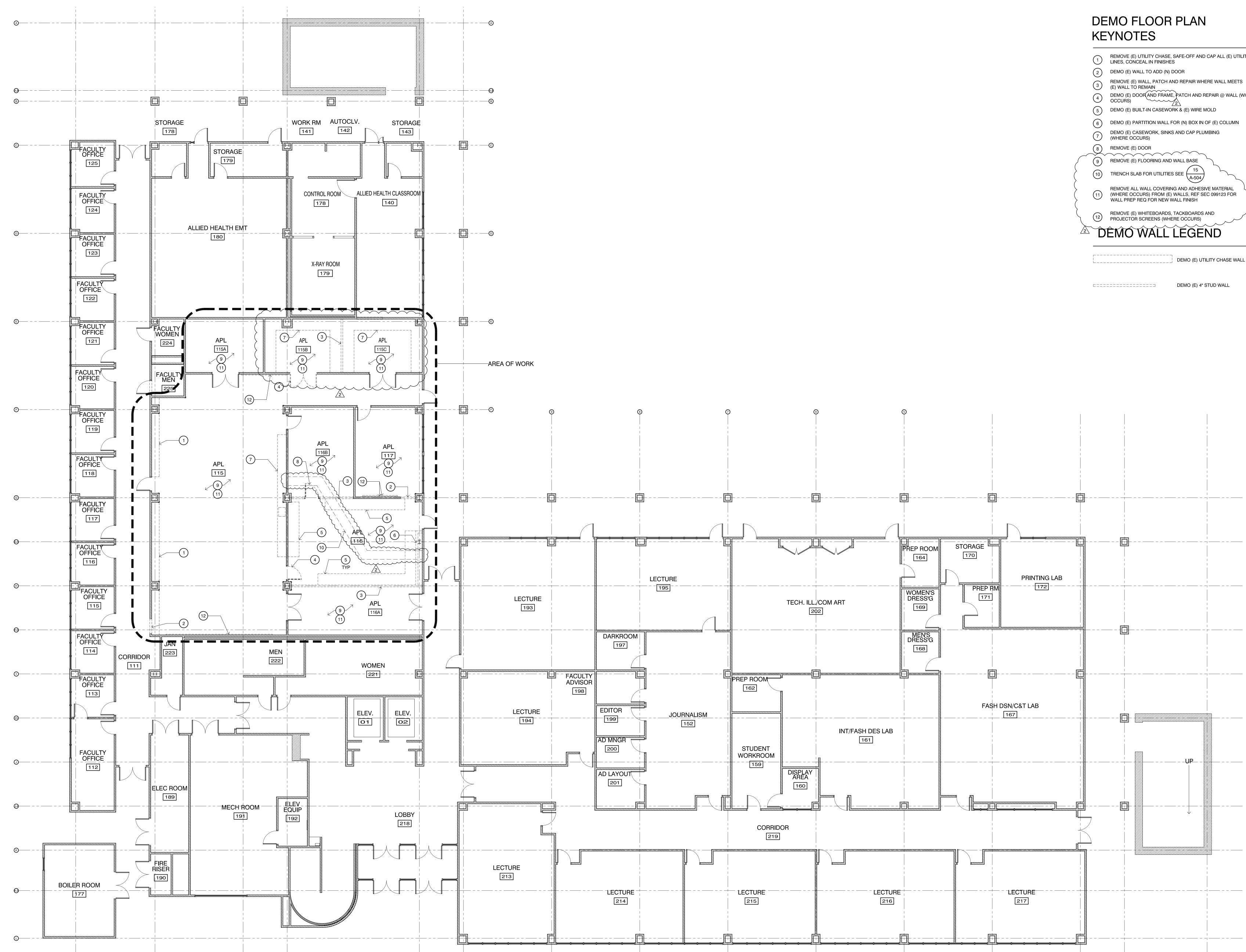
1 REMOVE (E) UTILITY CHASE, SAFE-OFF AND CAP ALL (E) UTILITY LINES, CONCEAL IN FINISHES REMOVE (E) WALL, PATCH AND REPAIR WHERE WALL MEETS 4 DEMO (E) DOOR AND FRAME, PATCH AND REPAIR @ WALL (WHERE OCCURS) (6) DEMO (E) PARTITION WALL FOR (N) BOX IN OF (E) COLUMN (1) REMOVE ALL WALL COVERING AND ADHESIVE MATERIAL (WHERE OCCURS) FROM (E) WALLS, REF SEC 099123 FOR WALL PREP REQ FOR NEW WALL FINISH
