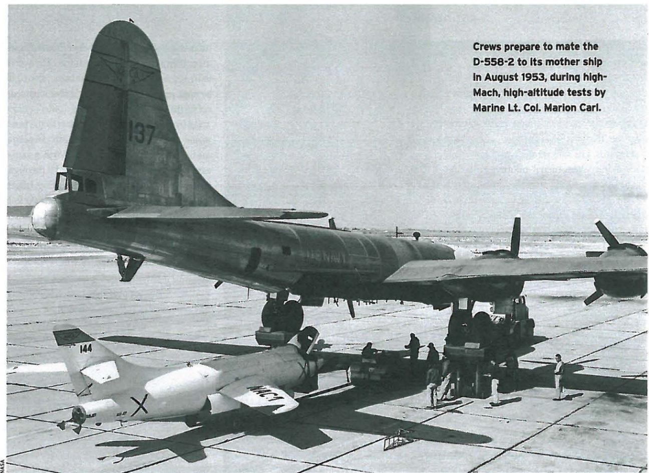
**Crews prepare to mate the D-558-2 to its mother ship in August 1953, during high-Mach, high-altitude tests by Marine Lt. Col. Marion Carl.**
